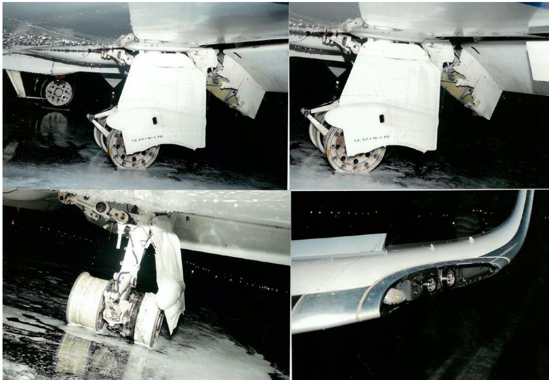
Fig:6 Damage to RH MLG and wing tip
