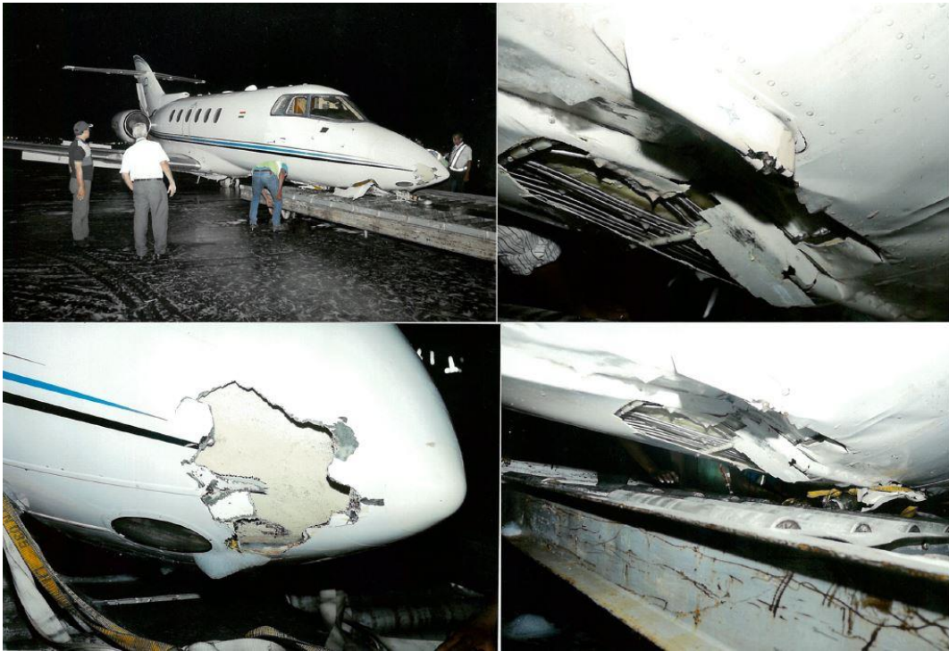
Fig: 2 Damage to radome and nose section
