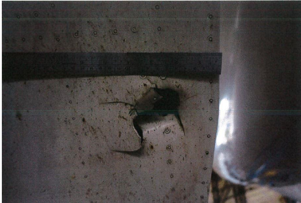
Fig:12 Damage to RH flap
