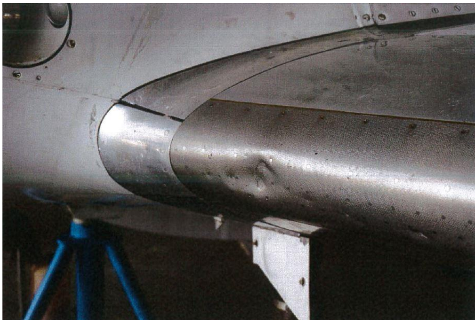
Fig:9 Damage to TKS panel of LH wing
