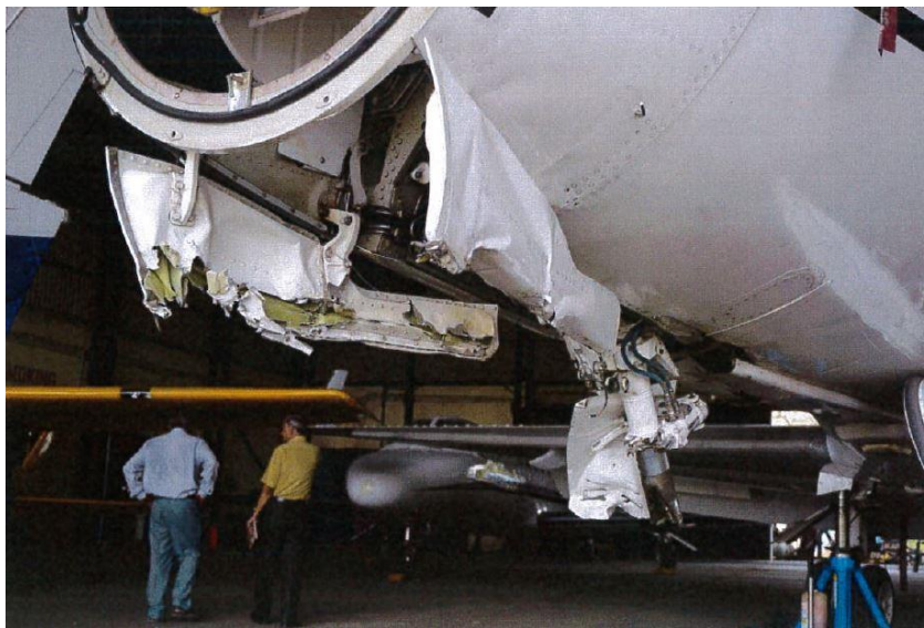
Fig:5 Damage to NLG and NLG door
