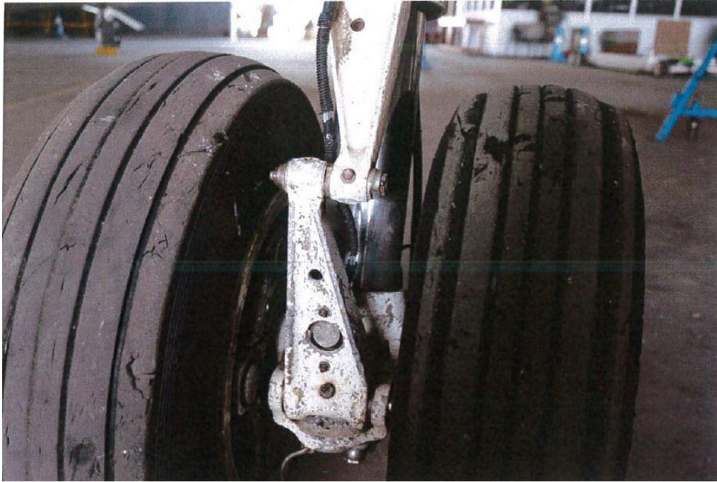
Fig:10 Damage to the RH MLG tyres
