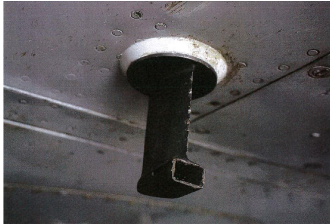
Fig:4 Damage to TAT probe
